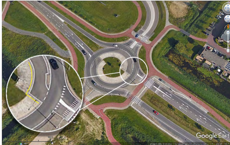
Figure 12. Photograph. Revised design used in the Netherlands for introducing the inner lane. (28)
